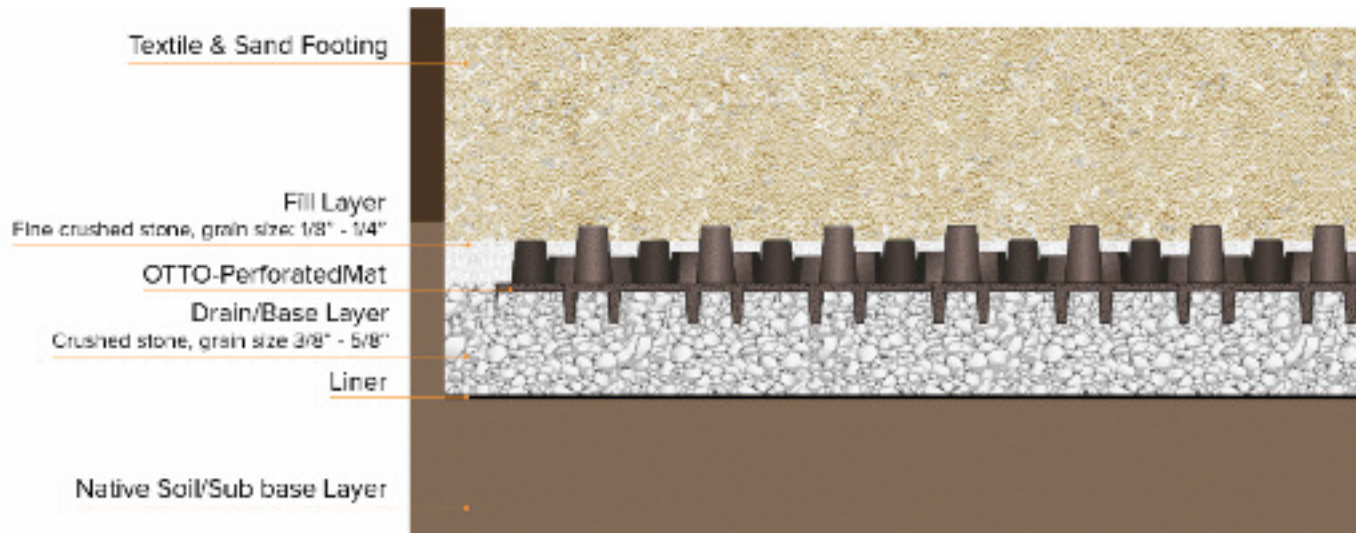
OTTO-PerforatedMats laid over a drainage layer
