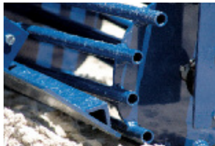
Smoothing bar and rollers smooth, compact, and finish the surface.
