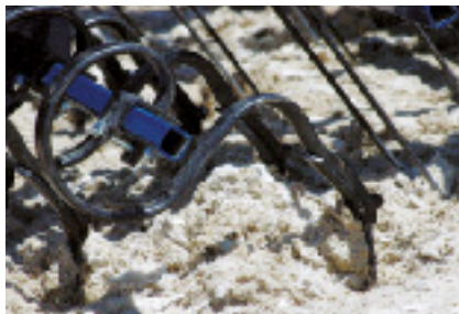
S-Tines & Coil Tines can be rotated to rip, lift, finish, and fluff.
